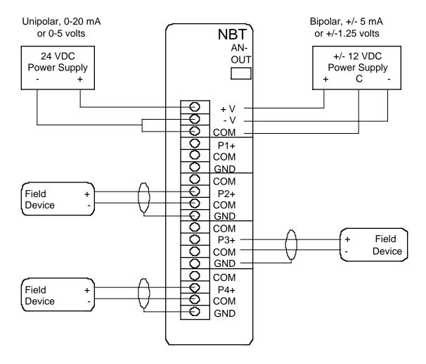
The analog output module requires a minimum of 16 VDC for unipolar operation. For bipolar operation, the power supply should be +/-12 VDC.
