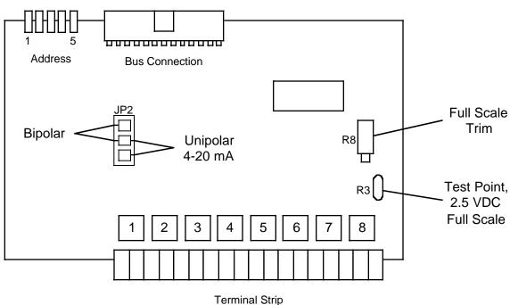
The four analog input modules (AIXA01-AIXA04) require +/-12 VDC (or 24 VDC) for full range operation. Load current for an analog input module is approx. 30 ma.
