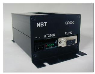
The SR900 is a reliable, wireless interface for most serial applications. The RF performance allows line of sight communications at distances over 15 miles. Non-line-of sight communications is also possible in many applications.
